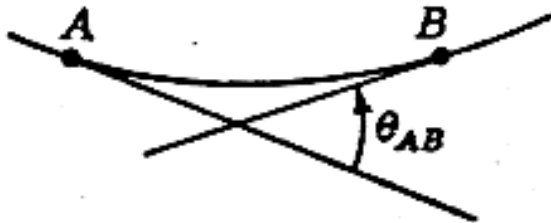
(a) Positive change of slope; \theta_{AB} is counterclockwise from left tangent
