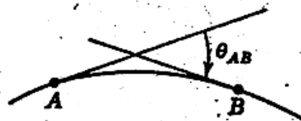
(b) Negative change of slope; \theta_{AB} is clockwise from left tangent
